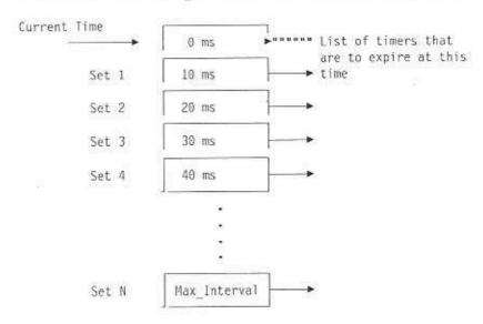
The basic idea behind the timing wheel technique is to sort the TCBs into different sets, depending upon the time of expiry. For example in Fig. 1, all TCBs for whom  $7.5ms \le B_T \le 10ms$ , are in Set 1, those for which  $10ms \le B_T \le 20ms$  are in Set 2 etc.. Furthermore, there is a pointer that points to the current time, and at every clock-
