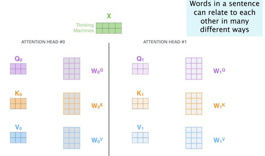
With multi-headed attention, we maintain separate Q/K/V weight matrices for each head resulting in different Q/K/V matrices. As we did before, we multiply X by the WQ/WK/WV matrices to produce Q/K/V matrices.
