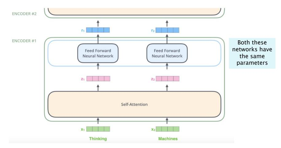
The word at each position passes through a self-attention process. Then, they each pass through a feed-forward neural network -- the exact same network with each vector flowing through it separately.
